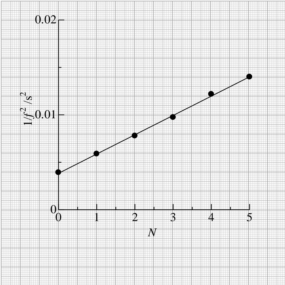
The additional quantities  $1/f^2$  are calculated in Table C.2. Then,  $\frac{M}{k'}$  and  $\frac{m}{k'}$  are obtained from the graph using the equation  $\frac{1}{f^2} = (2\pi)^2 \left( \frac{M}{k'} + \frac{m}{k'} N \right)$ .
