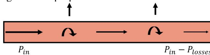
To first order, the average temperature gradient will be proportional to the average heat flow. Therefore, the temperature gradient will be proportional to
