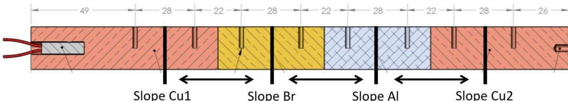
$$\kappa_{Brass} = \kappa_{Copper} \cdot \frac{\frac{2}{3}(\Delta T_{cu1}/\Delta x) + \frac{1}{3}(\Delta T_{cu2}/\Delta x)}{\Delta T_{Br}/\Delta x} = 115 \left[ \frac{W}{mK} \right]$$
