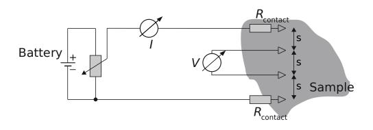
The curve *I versus V* represents the I - V-characteristics of the sample and allows the resistance of this sample segment to be determined. In the following we will only use the 4PP technique. To start, we will use the linear *equidistant* arrangement of four out of the eight probes (contacts) shown in the photograph.
