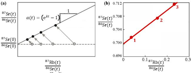
**Figure 1.2 (a)** The ratio  ${}^{87}$ Sr/ ${}^{86}$ Sr in different minerals at the time t = 0 of crystallization (open circles) and at present time (filled circles). (b) The isochron-line for three different mineral samples taken from a meteorite at present time.
