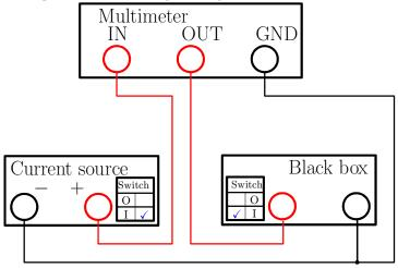
i. (1 pt) During charging of the capacitor from V=0 to  $V=V_{\rm max}$  we note that the output of the current source is constant  $(I_0=6.0\,{\rm mA})$  close to the precision of the multimeter. ii. (1.2 pts) Using the definition of differential capacitance, we can calculate the current through the capacitor in the black box from the time derivative of the voltage on the black box.
