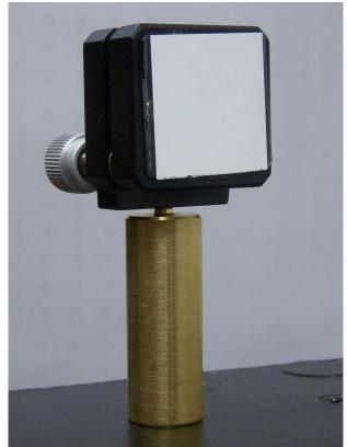
Mirror on a movable mount with two adjusting knobs and support post (LABEL B).
