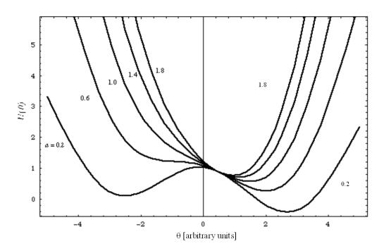
Figure 5: Graph of the function  $U(\theta) = \frac{a}{2}(\theta - \theta_0)^2 + \cos\theta$  (which is proportional to the potential energy of this problem) as a function of  $\theta$ , with  $\theta_0 \neq 0$ . The various curves correspond to different *a* values as labeled in the figure; smaller values of *a* (*a* < 1) correspond to the appearence of the bifurcation. In our case the parameter *a* is associated with the position *x* of the threaded rod.
