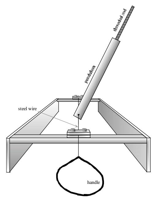
Figure 1: Sketch of the experimental apparatus when its rotation axis is horizontal.
