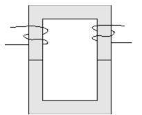
Figure 2: A transformer with a closed magnetic circuit.
