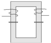
Figure 3: The ferrite cores with the two spacers in place.
