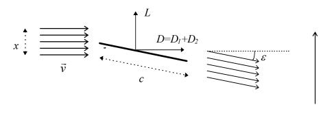
incident air wing section air leaving wing vertical(up)
