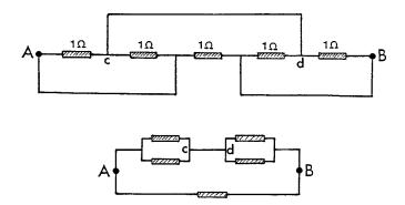
The equivalent drawing of the circuit shows that the resistance between point c and point A is  $0.5\Omega$ , and the same between point d and point B. The resistance between points A and B thus consists of two connections in parallel: the direct  $1\Omega$  connection and a connection consisting of two  $0.5\Omega$  resistances in series, in other words two parallel  $1\Omega$  connections. This yields
