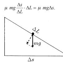
Adding up, we find that along the whole path the total work done by friction forces i  $\mu mg s$ . By energy conservation this must equal the decrease mg h in potential energy of the skier. Hence
