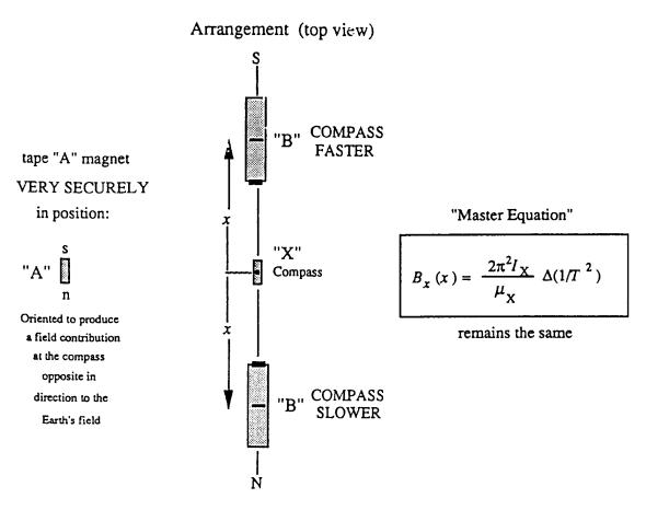
Use only <u>partial</u> buckout --(slow natural oscillations typically by a factor of 2) In working at a given distance x,  $\Delta(1/T^2)$  must be constant (independent of the "bucking").
