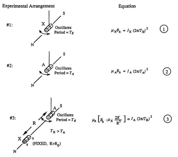
Note that the X magnet (positioned at a distance R which is somewhat larger than the turn-around distance  $R_0$ ) is being used here to <u>slow</u> the oscillations of the A magnet on the compass.
