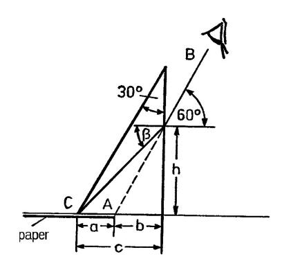
Place edge C of the prism on edge A of a sheet of paper and look along the prism hypotenuse at edge A so that your direction of sight B-A and the table surface form an angle of 60°. Then shift the prism over the edge of the paper into the position shown, such that prism edge C can be seen inside the prism collinear with edge A of the paper outside the prism. The direction of sight must not be changed while the prism is being displaced.
