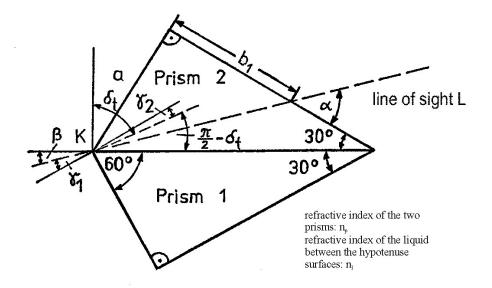
If the refractive index of the prism is known (see part a) the refractive index of the liquid may be calculated as follows:
