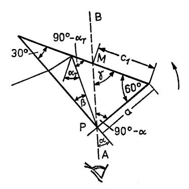
Draw a straight line A – B on a sheet of paper and let this be your line of sight. Place the prism with its rectangular edge facing you onto the line (at point P on the line). Now turn the prism in the direction of the arrow until the dark edge of total reflection which can be seen in the short face of the prism coincides with the 90° edge of the prism. Mark a point M and measure the length  $c_1$ . Measure also the length of the short face of the prism.
