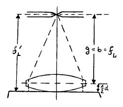
The distance between pencil point and mirror has to be determined with an accuracy, which enables one to state  $f_L$  with a maximum error of  $\pm 1 \%$ . This is accomplished either by averaging several measurements or by stating an uncertainty interval, which is found through the appearance of parallaxe.
