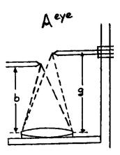
In order to have object and image in focus at the same time, they must be placed at an equal distance to the eye. In this case object distance and image distance are the same and the magnification factor is 1.
