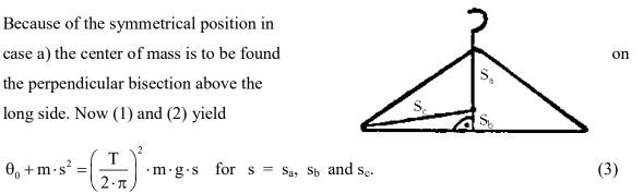
because all periods of oscillation are the same. This quadratic equation has only two different solutions at most. Therefore at least two of the three distances are equal. Because of  $s_c > 21 \text{ cm} > s_a + s_b$ , only  $s_a$  and  $s_b$  can equal each other. Thus we have
