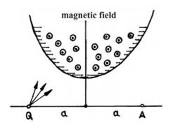
$(\overline{QA} = 2 \cdot a)$ . The trajectories of the ions are symmetric to the middle perpendicular on  $\overline{QA}$ .
