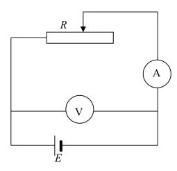
Sliding the contact along the rheostat sets the current I supplied by the source. For each value of I the voltage U across the source terminals is recorded by the voltmeter. The power dissipated in the rheostat is:
