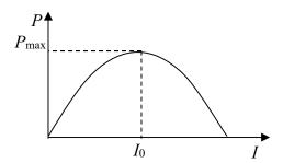
If the current varies in a sufficiently large interval a maximum power  $P_{\text{max}}$  can be detected at a certain value,  $I_0$ , of I. Theoretically, the P(I) dependence is given by: (5.
